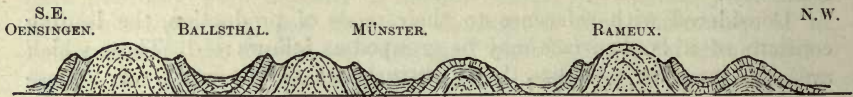
Fig. 500.—Symmetrical Flexures of Swiss Jura (the ridges coinciding with anticlines and the valleys with synclines).
